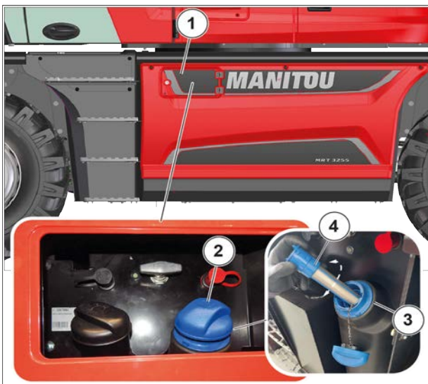
Figure 226: Checking and cleaning the DEF tank filler filter
